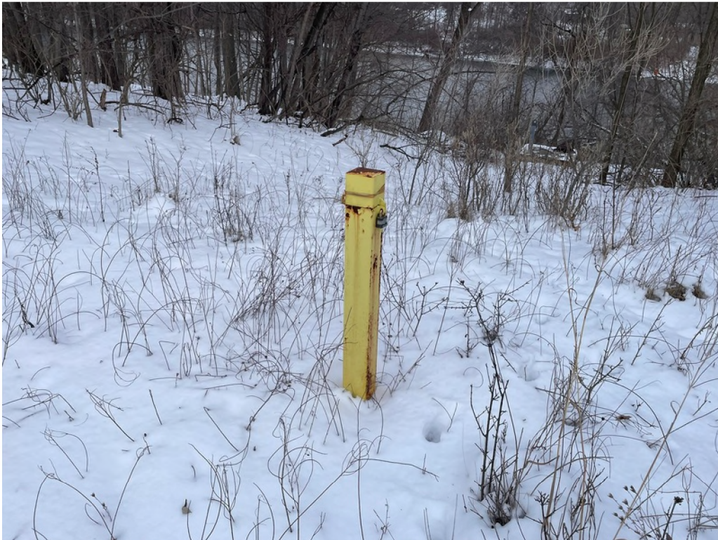
Piezometer in the northeastern portion of subject property
